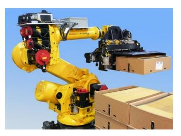
**Benefits:** Remtec's Robotic Magazine Loader can help you realize the full potential of your cartoning operation. For cartoning rates in excess of 250 cpm and with case loads up to 100 lbs, this is the perfect solution for high-rate ergonomically challenging magazine loading applications
